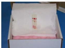
■ Lay the test plate down on a flat bed scanner for a quick scan and loading to database\* or send it to [info@alpha-cat.org](mailto:info@alpha-cat.org). The colors on the plate will fade over time. The plate will turn reddish as it is exposed to light and air over a short period of time. Do the reading of the dots and scanning between 4 and 8 minutes after the test plates are coming out of the developing chamber.
